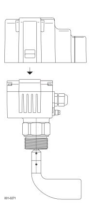
After the electrical connection push on the weather protection hood and press it down until the laterally knobs snap in.
