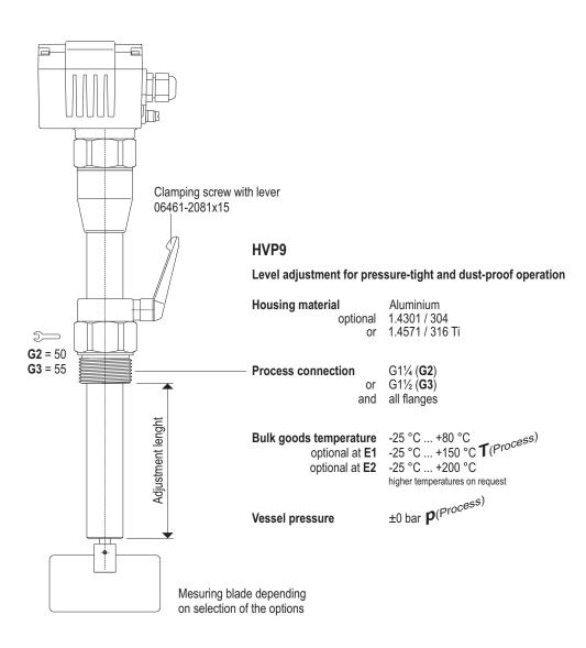
ATTENTION! At temperatures above +60 °C change the level adjustment only in cold condition or carry the appropriate safty gloves.
