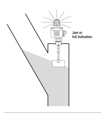
Selection of lamp functions for the large signal lamp H8
