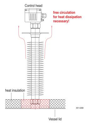
If it is mounted horizontal or inclined the device may be installed in a vessel without heat insulation.
