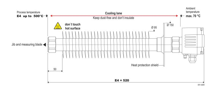
The Technical Data presented here are to be considered as maximum values, relating only to the equipment described herein. Depending on the selection of options and instruments used, these data must be considered or reduced correspondingly.
