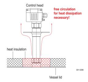
If it is mounted horizontal or inclined the device may be installed in a vessel without heat insulation.
