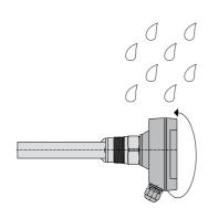
The cable glands must always point downwards to prevent moisture seeping inside the housing. If the housing is not in the correct position after the probe has been firmly screwed into the bin wall, proceed as follows:
