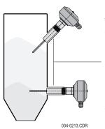
Due to the low installation depth the **VF62** is although suitable for the use in small bins.
