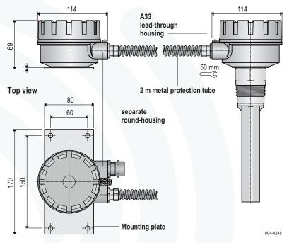
With the separate round-housing the electronic will be mounted remote from the probe.
