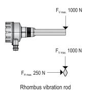
Due to the special shape of the Rhombus vibration rod, it is very robust and able to resist high forces up to 1000 N in vertical direction.
