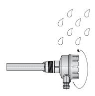
The cable glands must always point downwards to prevent moisture seeping inside the housing. If the housing is not in the correct position after the probe has been firmly screwed into the bin wall, proceed as follows:
