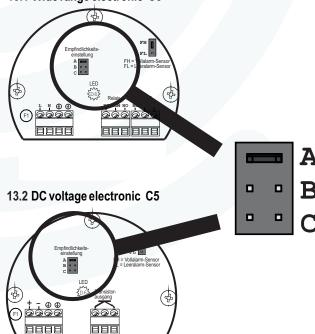
Adjustment by jumper at A-B-C
