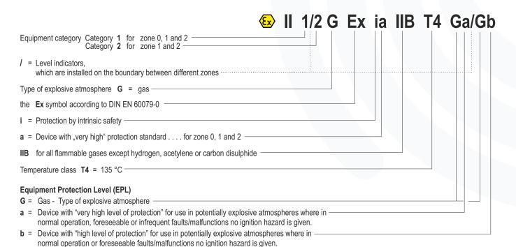
The "very high" protection standard of the devices permits although the use complete in zone 20 and zone 0. Please request further information if needed.
