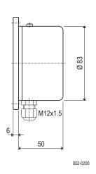
\* Hole-Ø in the vessel max. 80mm
