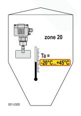
The ambient temperature Ta defines the maximum operating temperature of the indicators. Inside the vessel this can be the ambient and/or the bulk goods temperature and therefore the process temperature.
