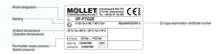
Note: The X behind the certification number indicates special conditions for the safe application of the equipment in the appendix to the EU-type examination certificate
