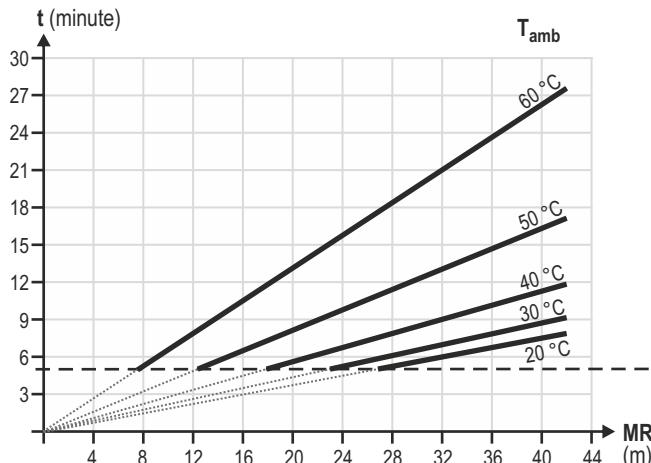
The minimum time ( $t_{\text{minute}}$ ) for one measuring cycle (time between two measurements) is dependent on the ambient temperature ( $T_{\text{amb}}$ ) and the measuring range ( $MR_{\text{meter}}$ ) and must not be undershoot in all types of measuring.
