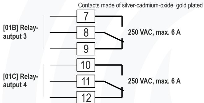
The rest position matches with the position of the relays without power supply.
