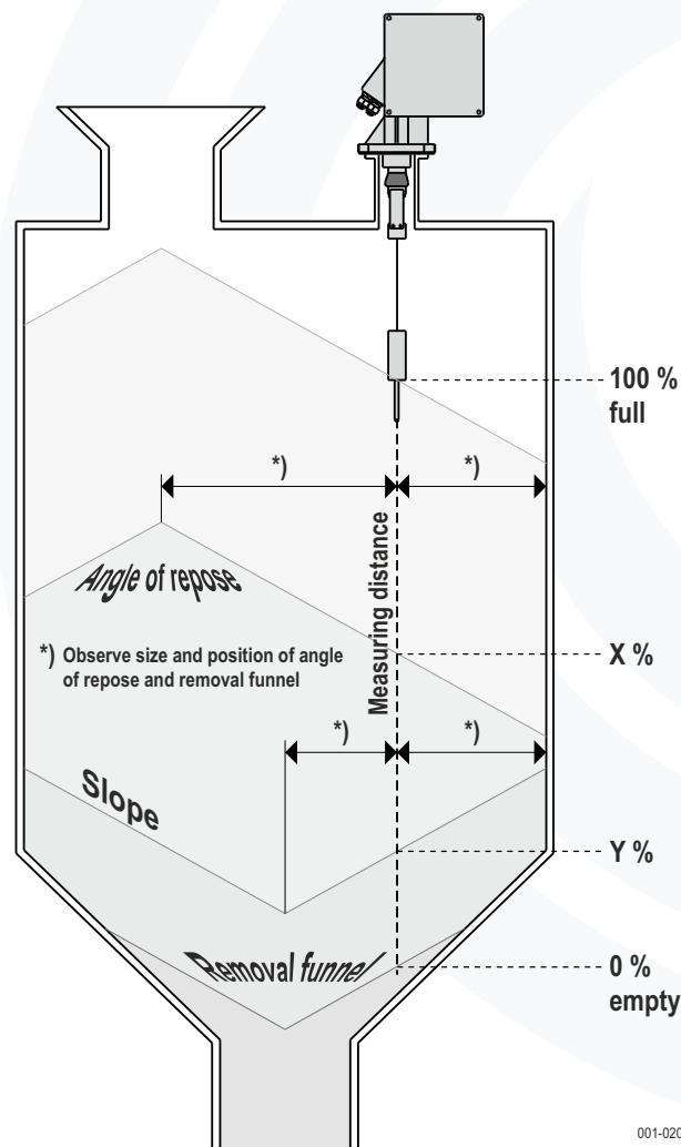
During the up and down movement of the sensing weight the relay output of the LF20 can additionally emit pulses according to the length of the rolled out measuring tape. These pulses can be recorded by a process control system or an electro mechanical counter.
