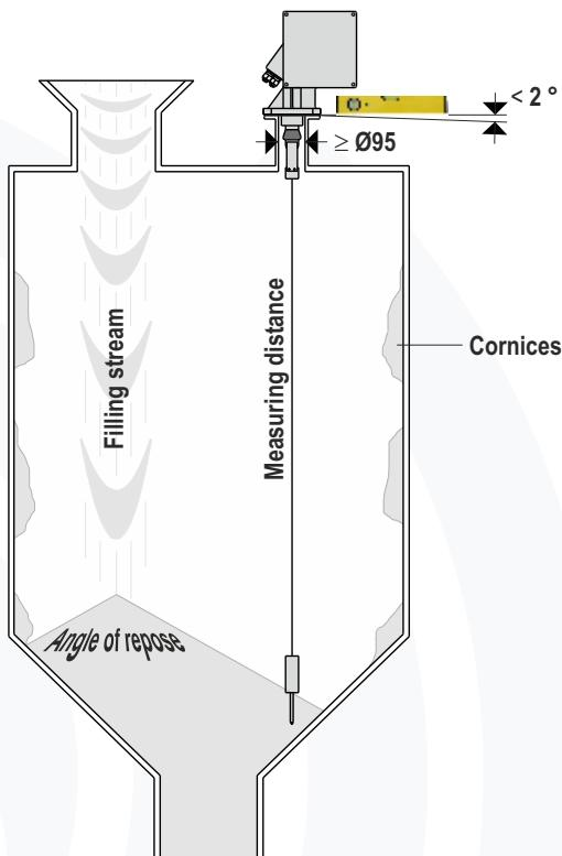
Select the mounting location on the bunker or silo roof in such a way that falling product during filling or collapsing cornices cannot spill the sensing weight and cannot damage the measuring tape.
