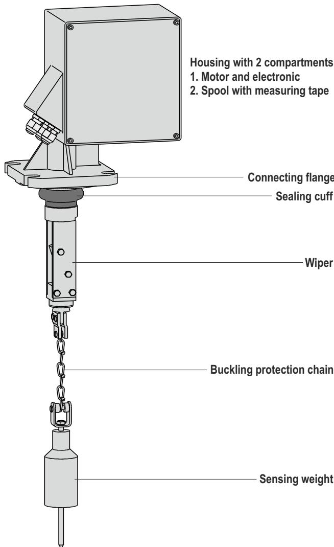
Sensing weight has to be suitable for the chemical characteristics of the bulk good and the process temperature within the bunker or silo.
