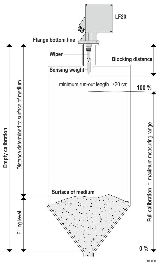
The measured value is the distance between the flange bottom line and the surface of the medium minus the block distance.
