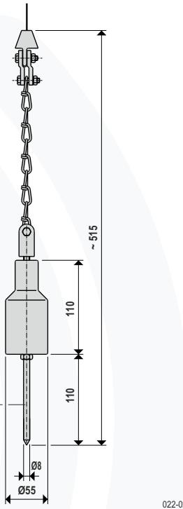
The spike avoids slipping or tilting of the sensor weight on a steep bulk surface.
