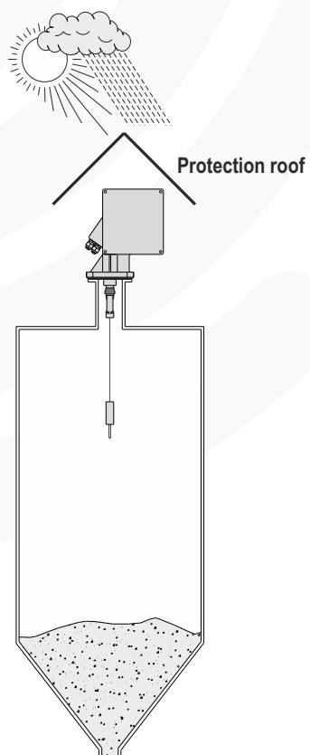
For use in external areas being exposed to climatic conditions we recommend the weather protection hood or an additional protection roof.
